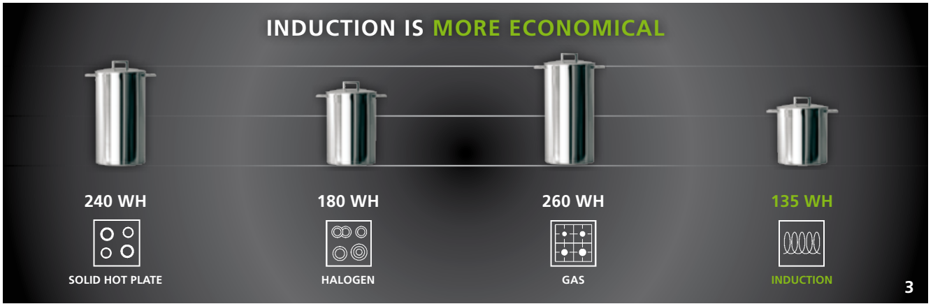
Consumption in Watt hours for heating up 1 litre/1.1 quarts of water in a pot with 18 cm/7.1" diameter on an 18 cm/7.1" zone from 18°C/65°F to 98°C/210°F
